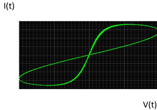
Fig 3 : Memristor Hysteresis Characteristic
