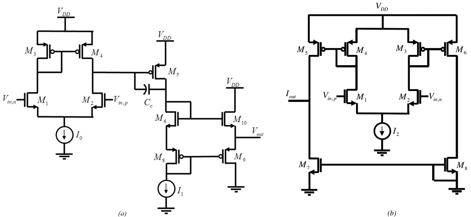
Figure 5- (a) Schematics of OpAmp1, 2-stage differential OpAmp with push-pull buffer, (b) Schematics of OpAmp2, transadmittance (TA)
