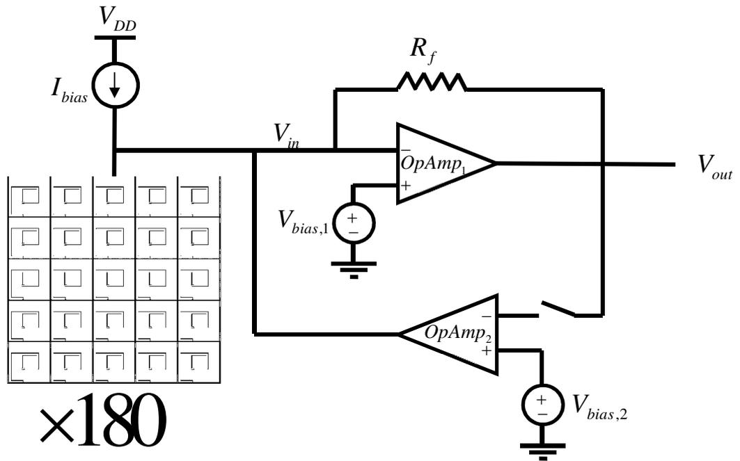
Figure 4- Read out integrated circuit structure
