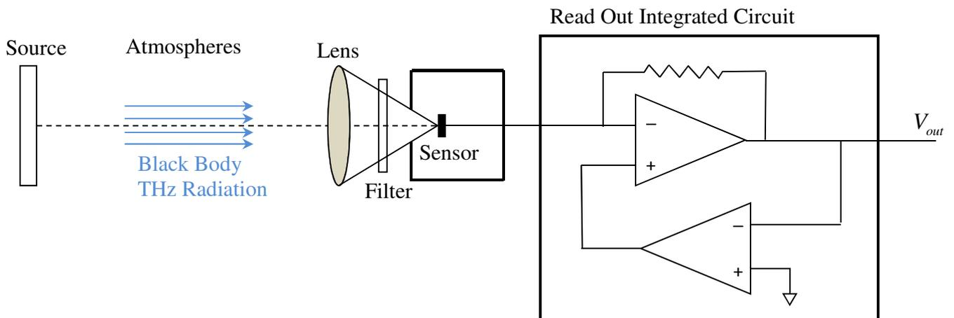
Figure 1 – THz sensor and read out circuit process diagram
