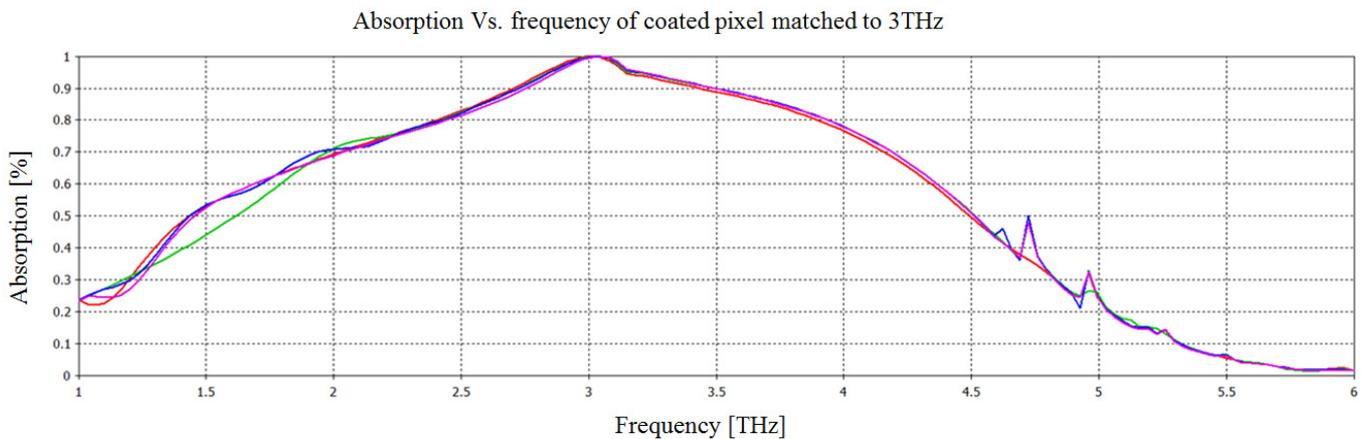
Figure 3 – Diagram of pixel 'Q' with Ti coating matched to 3 THz with 100% absorption and large BW
