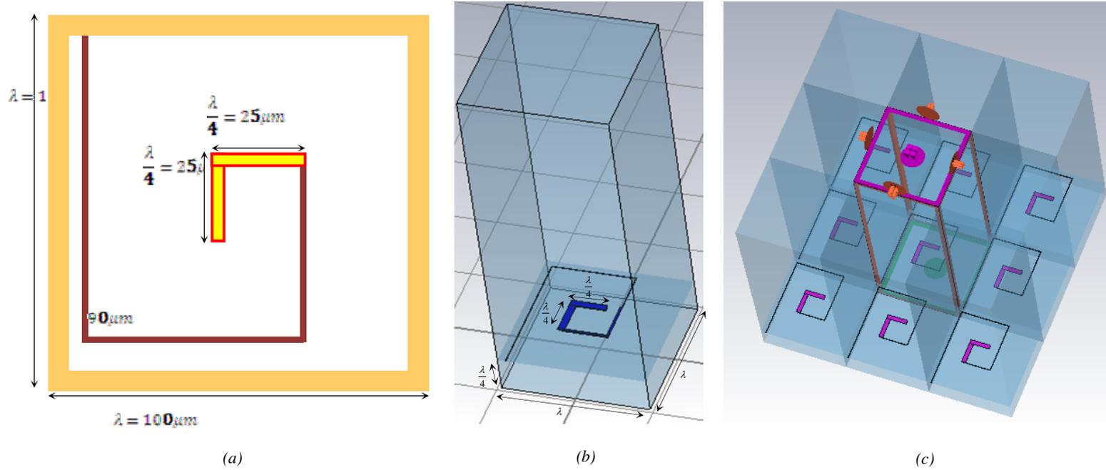
Figure 2- (a) pixel 'Q' with 2 series connected transistor, matched to  $\lambda = 100 \mu\text{m}$  ( $f = 3\text{THz}$ ). (b) Full pixel 'Q' view, pitch is  $\lambda$ , antenna matched to  $\frac{\lambda}{4}$  and optical cavity matched to  $\frac{\lambda}{4}$ . (c) Periodic array of pixel 'Q'.
